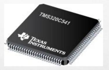
TO IMPLEMENT SDR, HIGH-SPEED DSPS AND FPGAS, ARE PRIMARILY USED SO AS TO MEET ABUNDANT BASEBAND PROCESSING DEMANDS OF SDR
